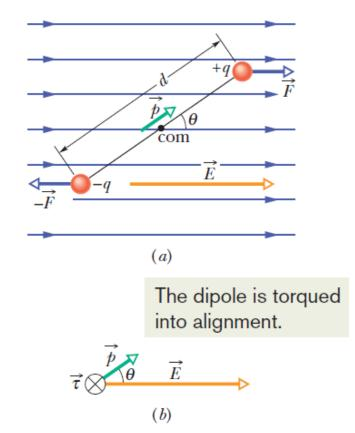
Fig. 22-19 (a) An electric dipole in a uniform external electric field  $\vec{E}$ . Two centers of equal but opposite charge are separated by distance d. The line between them represents their rigid connection. (b) Field  $\vec{E}$  causes a torque  $\vec{\tau}$  on the dipole. The direction of  $\vec{\tau}$  is into the page, as represented by the symbol  $\otimes$ .
