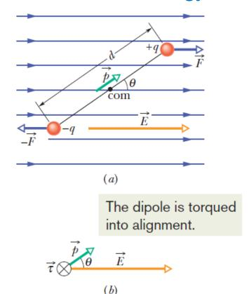
Fig. 22-19 (a) An electric dipole in a uniform external electric field  $\vec{E}$ . Two centers of equal but opposite charge are separated by distance d. The line between them represents their rigid connection. (b) Field  $\vec{E}$  causes a torque  $\vec{\tau}$  on the dipole. The direction of  $\vec{\tau}$  is into the page, as represented by the symbol  $\otimes$ .
